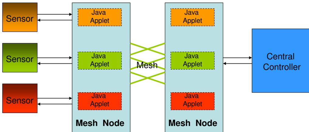
Figure 2: An object-oriented, open-systems architecture for a flexible wireless mesh-based sensor system. Intelligent mesh nodes control sensors via downloadable applets and handle the archiving, compression, and routing of sensor data. A central controller distributes applets to govern sensor behavior and requests sensor data on an as-needed basis.
