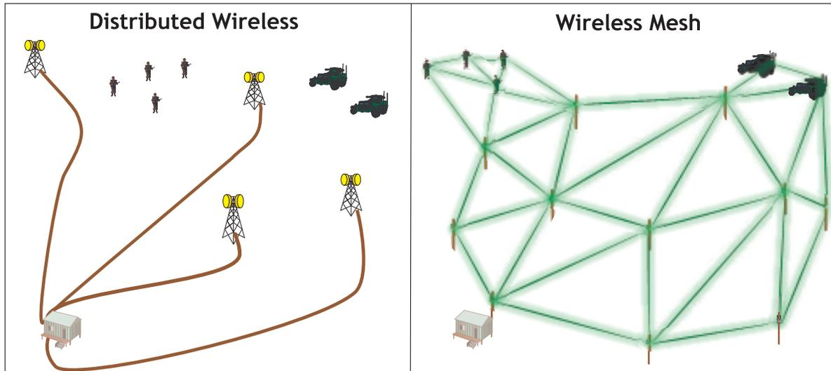
**Figure 1:** A traditional distributed wireless topology requires miles of cable and large fixed antennae, while a mesh topology relies on peer-to-peer communication between low-cost, relatively low power radios. Mobile mesh nodes mounted on vehicles or carried by personnel are instantly integrated into the mesh
